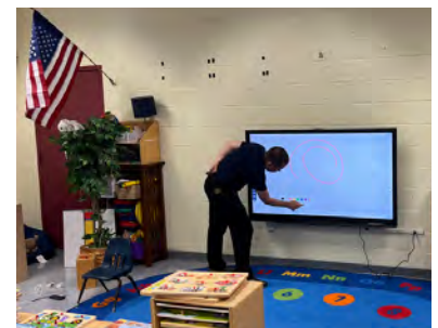
An interactive panel installed in a pre-school classroom. Note they are installed much lower for Pre-K and K so students can reach them.
